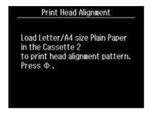
7. Press the  $\diamondsuit$  start button to print an alignment sheet.
